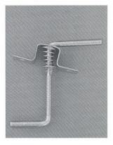
First slide the washer on the end closest to the notch. The spring goes on the lever next, make sure that the narrow end will be next to the washer. The last step is to slide the lever bracket on to the lever so that it partially encloses the spring as shown in the picture.
