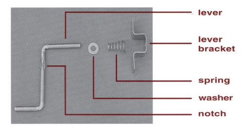
The four components of the door latch that will need to be assembled are: lever, washer, spring and lever bracket. The lever is notched on the middle section to act as a stop for the other components.
